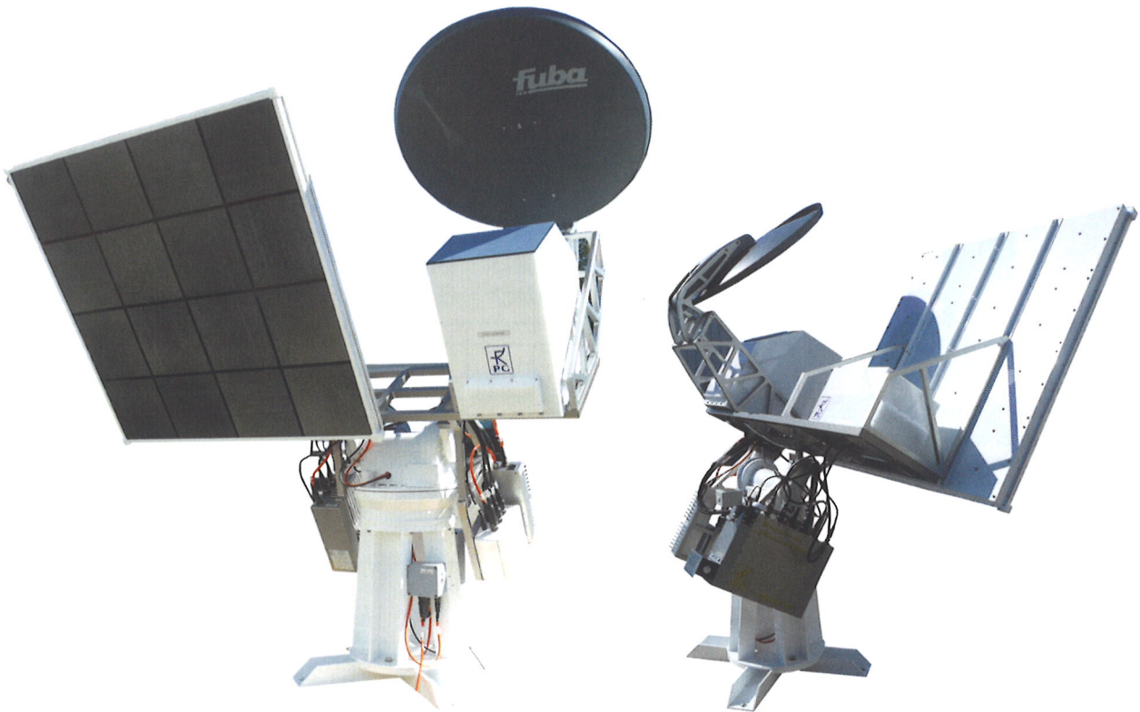
Typical combination: L-band (front view, left) and 6.925/10.65 GHz packages (front view, right).
