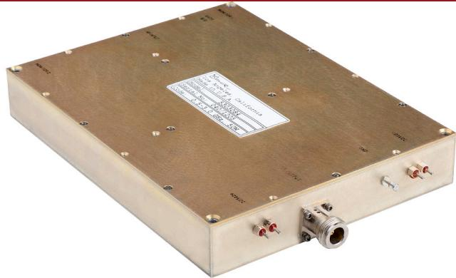
The building block of any high power RF/Microwave system is the amplifier module.
